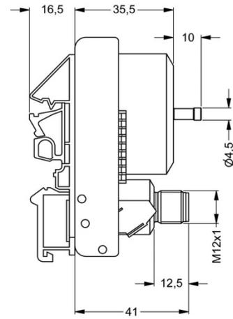
hose connection for flexible hoses  $\varnothing 4$  mm
