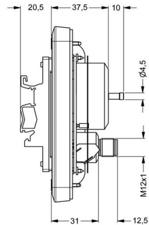
hose connection for flexible hoses  $\varnothing 4$  mm
