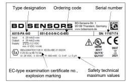
Fig. 1 example of manufacturing label
