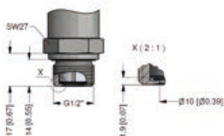
G1/2" semi-flush DIN 3852 ( p_N from 0.4 up to 60 bar)
