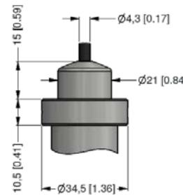
cable outlet with PVC cable (IP 67)<sup>4</sup>
